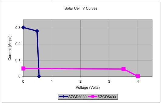
In either case, the point you want to operate at to get the most power is at the Imp, Vmp values. To operate here, you choose the resistance (R = V / I) to be at that point. This is called the characteristic resistance of a solar cell.
