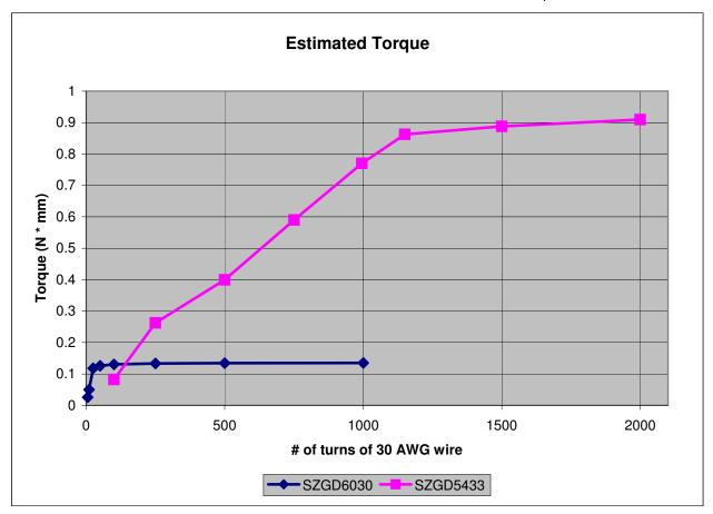
Less turns than the calculated optimum results in less torque. More turns doesn't get any more torque.
